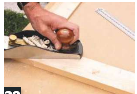
30 True up front and rear faces of doors with bench plane. Check surfaces with steel straightedge
